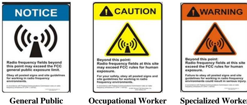
All signage shall be of made of weather, corrosion, and ultra-violet (UV) resistant materials.
