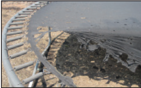
Embers destroyed this trampoline.
