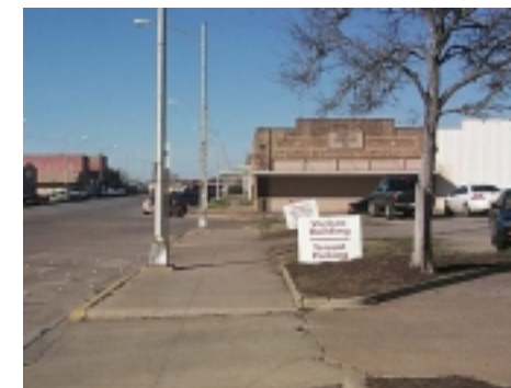
Extensive curb cuts interrupt the network of sidewalks and landscaping, decrease the safety for pedestrians and challenge vehicular safety.
